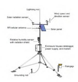
Image 6.2: Weather Station: Representative Image and Diagram
